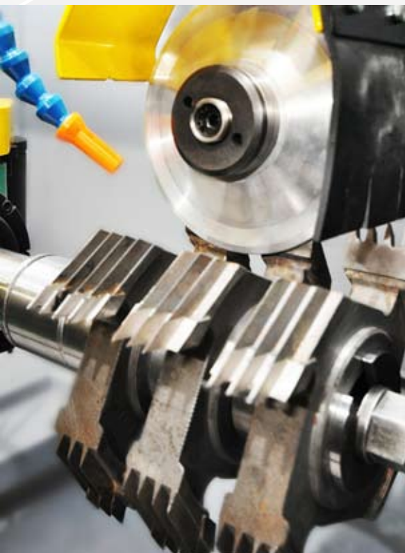
Sharpening cutters for finger joints
