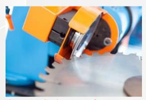
Sharpening the clearance surface
