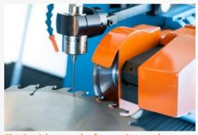
The Renishaw probe for precise tooth measurement
