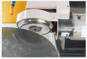
Sharpening the clearance surface and bevelling
